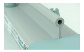
The divider used on all Meech pulsed DC bars is an essential feature that ensures good operation in dirty, factory environments. To maximise the interval between cleaning the 971IPS-30 bar features a divider to increase the surface tracking distance between the two rows of high voltage pins. It is important to clean this area during cleaning operations.
