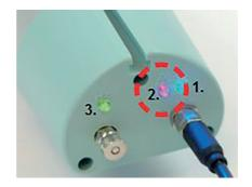
When the equipment powers on, the (1.) Blue LED will illuminate and the (3.) Hz LED will start to flash red and green in time with the Hz setting. If (2.) Warning LED starts to flash or is solid red, check the ion level with the BarMaster.
