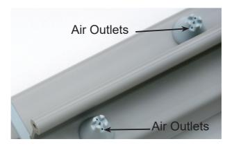
Whilst the long range performance of the Hyperion 971IPS-30 is excellent, some installations can require the use of air assistance to get full control of the static. This can either be by increased speeds of decay and/or by increased ionisation range. Air outlets either side of the emitter pin ensure that the integrated air-boost is extremely efficient. Each 971IPS-30 bar is supplied with a 6mm push-fit air fitting pre-installed.
