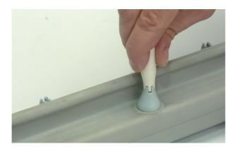
After prolonged use, perhaps after several years, the emitter pins may become worn and require replacement. Bags of replacement pins are available from Meech and are supplied with a special insertion tool.
