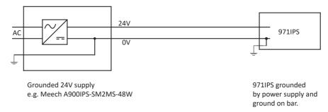
Connection using an ungrounded 24V DC power supply.
