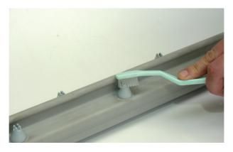
To maintain good performance, regular cleaning of all ionising bars is required. The open design of the 971 emitter head allows for easy and effective cleaning with a brush, making removal unnecessary. A dry toothbrush is ideal.
