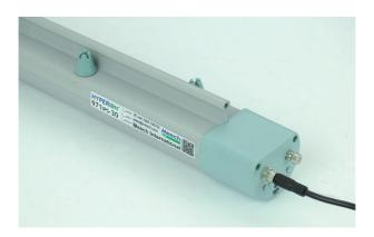
The profile of the Hyperion 971IPS-30 bar is rounded, with minimal dirt traps, making it useful for cleanroom applications. The bar has good rigidity, allowing it to span wide widths. Mounting is by M4x20 T bolts in a slot at the rear of the bar.
